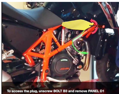
Then augmented reality takes over to guide the repair technician step by step.
