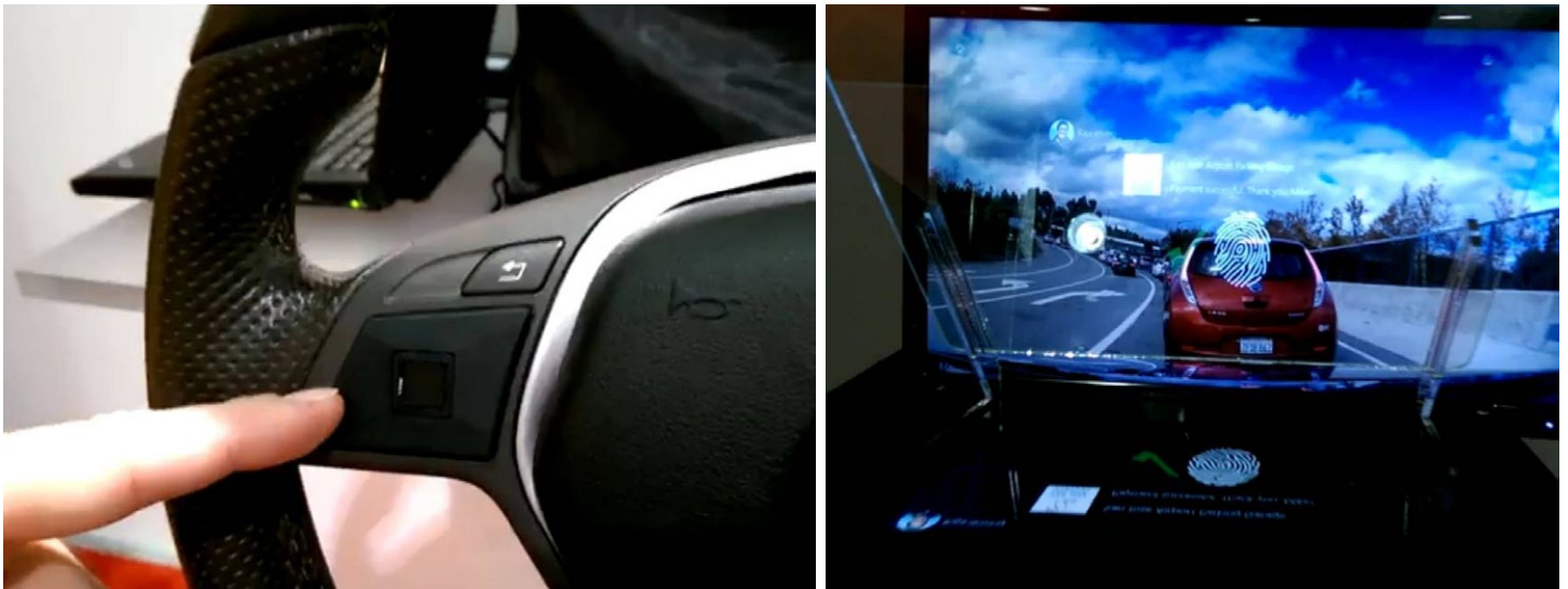
Synaptics' 8x8mm Natural ID fingerprint sensor integrated on the directional pad (D-Pad) of a steering wheel.
